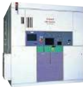
Canon FPA-5500iZa stepper Approximate dimensions: 7.5 x 11.1 x 8.5 ft. (W x D x H)
